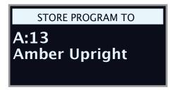
To select a different store location use the dial and/or the PROGRAM 1-5 buttons. A program can also be stored to one of the Live program locations by pressing the LIVE MODE button and then selecting the desired Live program. The program at the selected
